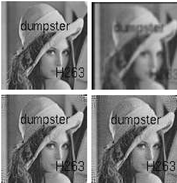
Figure 3 - Top Left, the ideal image. Top Right, bilinear interpolation. Bottom Left, LS solution. Bottom Right, PSGD solution.
