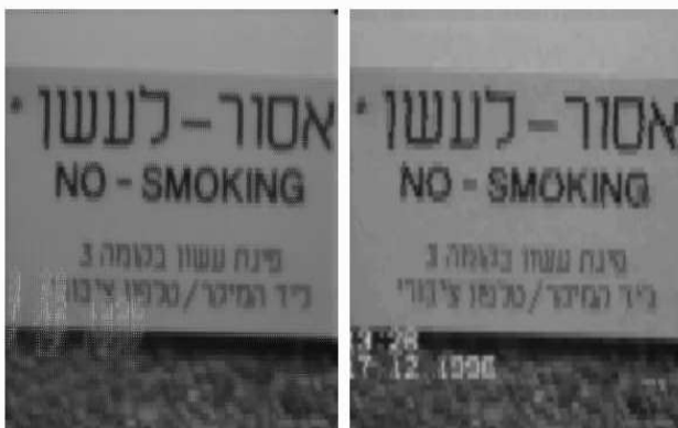
Figure 4 - Super Resolution reconstruction from a real video sequence. Left - PSGE result. Right - Bilinear interpolation.
