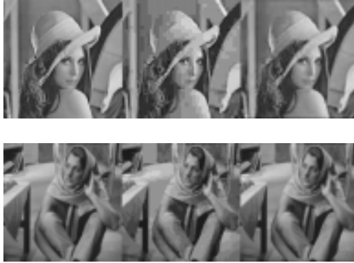
Fig. 1. Original image (on the left) JPEG compressed–decompressed image (middle), and down-scaled–JPEG compressed-decompressed and up scaled image (right). The down scaling factor - 0.5. In both cases, the compression ratio is 40. The MSE in the upper row is 219.5 (left) and 193.12 (right). Similarly, in the lower row: 256.04 (left) and 248.42 (right).
