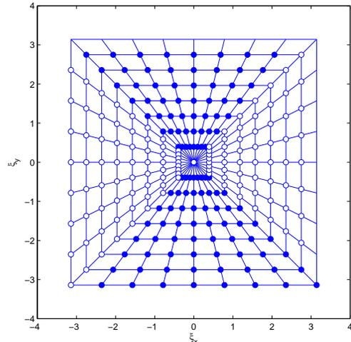
Figure 1: The pseudo-polar grid and its separation into BV and BH coordinates ( $N = 8$ ).
