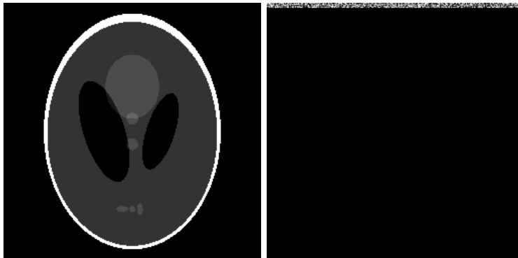
Figure 3: An example of a piecewise constant image: the 256 \times 256 Shepp Logan phantom (left); and an image with the same cosparsity, \ell = 128014 , but whose cosupport is associated with an empirically maximum subspace dimension (right).
