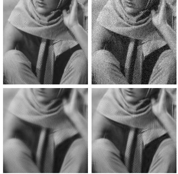
Figure 8. Denoising results (using iterative-shrinkage) of a 256 \times 256 slice of Barbara (for \sigma_n = 20 ). From left to right and top to bottom: Original; Noisy ( PSNR = 22.10dB ); Iteration no. 1 ( PSNR = 27.03dB ); Iteration no. 2 ( PSNR = 29.46dB ).
