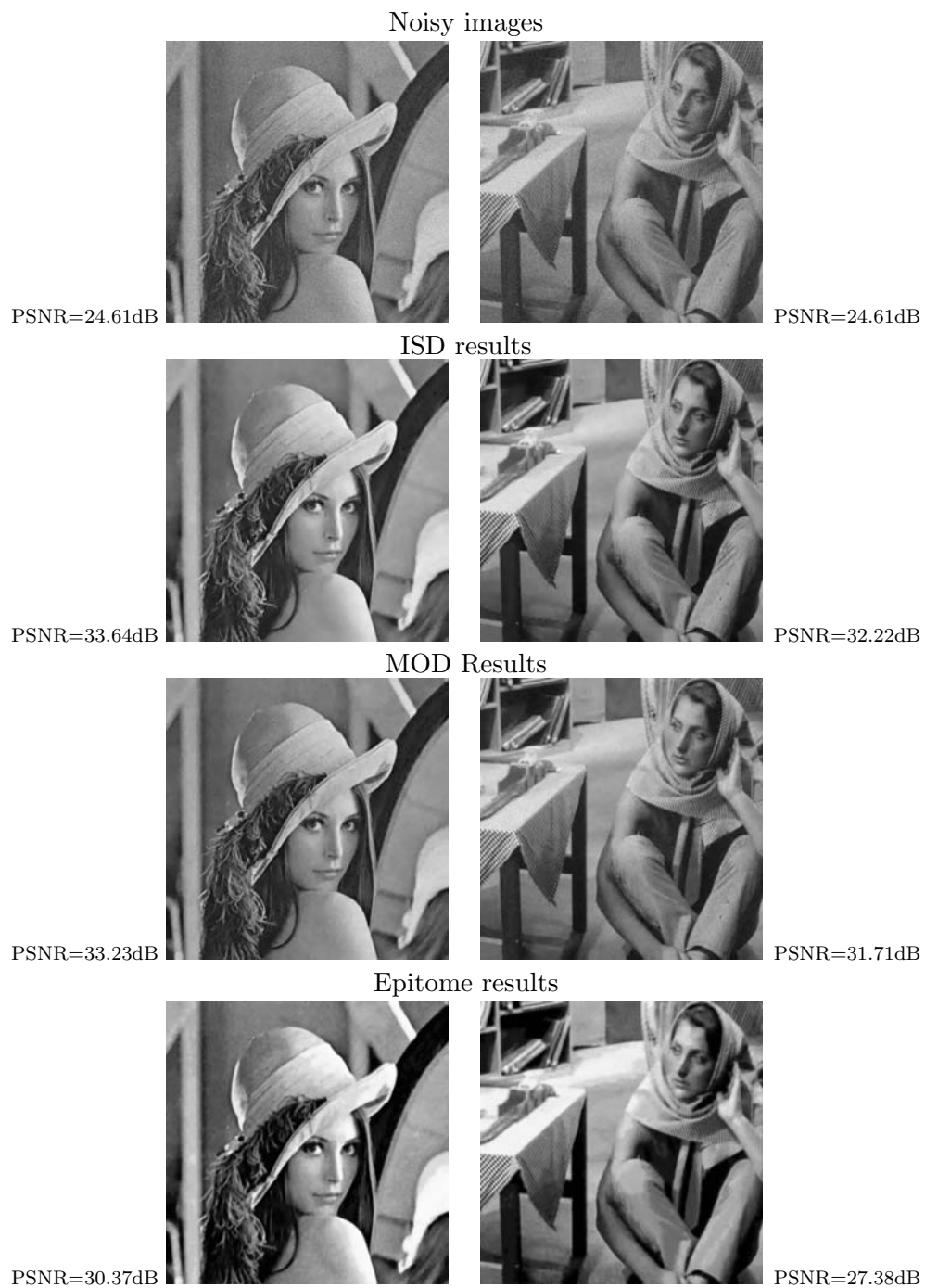
Figure 8. Selected denoising results. These results refer to noise power \sigma = 15 , showing the noisy image, the ISD, the MOD, and the epitome denoising results.
