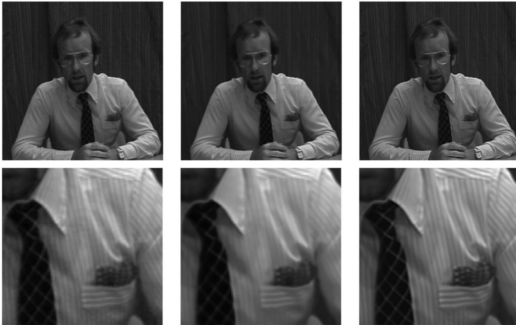
Fig. 2. Original “Trevor” sequence. Left: Interpolated image. Middle: Interpolation, followed by NLM processing and deblurring. Right: Proposed algorithm. Bottom row offers a close-up of a portion of the images.
