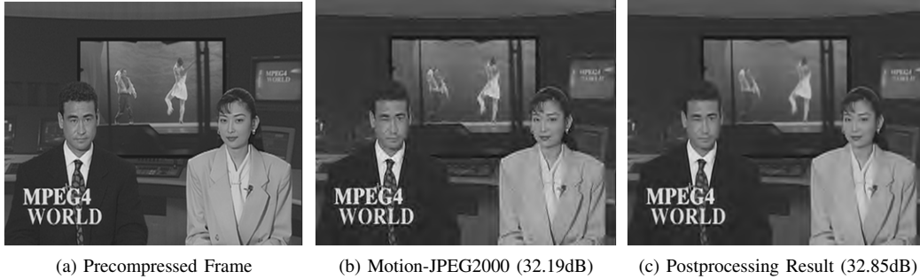
Fig. 2. Reconstruction of News (CIF) from Motion-JPEG2000 compression at 0.27bpp.
