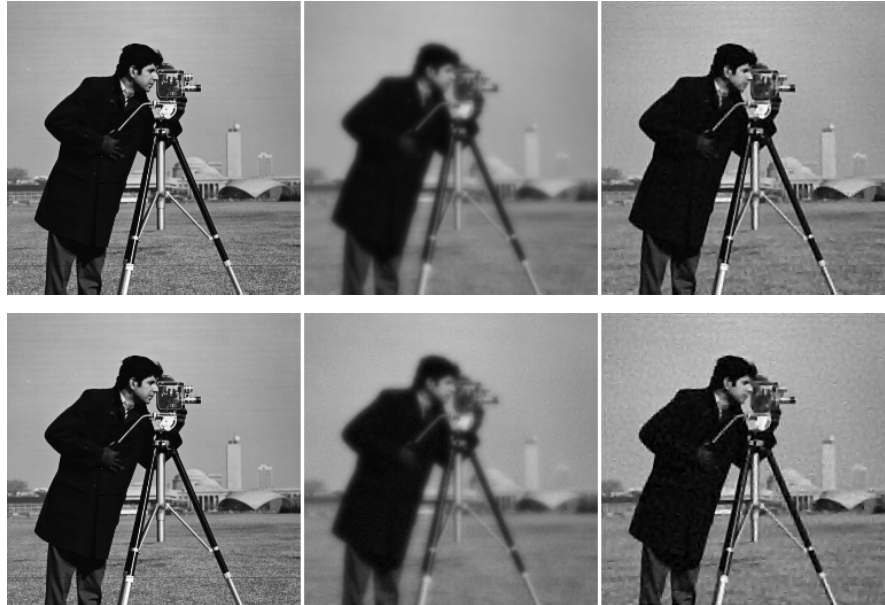
Figure 4. Deblurring results with the PCD-SESOP0 algorithm: Original image (left), measured blurry and noisy image (middle), and restored (right). Top images refer to the experiment with \sigma^2 = 2 , and the bottom ones for \sigma^2 = 8 .
