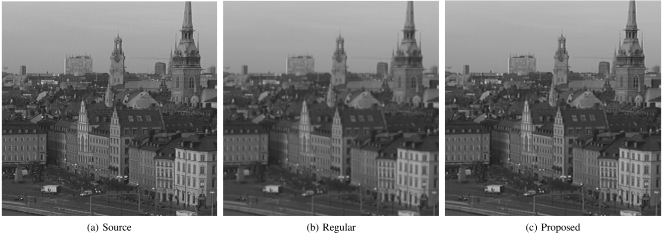
Fig. 4. Coding a group of 10 frame from the 'Stockholm' sequence (spatial portion of 480x480 pixels). (a) The third source frame. (b) the rendered frame using regular compression (28.29 dB at 2.37 bpp). (c) the rendered frame using the proposed compression (29.45 dB at 1.34 bpp).
