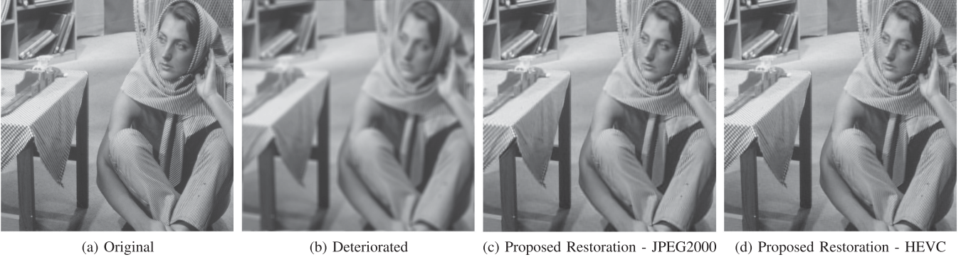
Fig. 8. The deblurring experiment (settings #2) for the Barbara image ( 512 \times 512 ). (a) The underlying image. (b) Degraded image (22.49 dB). (c) Restored image using Algorithm 3 with JPEG2000 compression (25.18 dB). (d) Restored image using Algorithm 3 with HEVC compression (27.72 dB).
